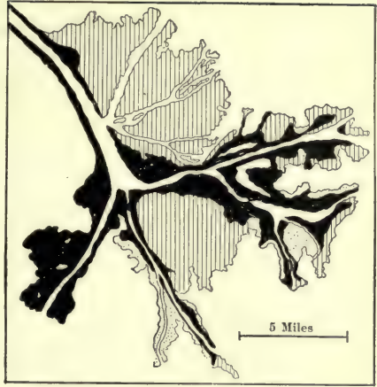
FIG. 142.—Map of the “passes” of the lower Mississippi delta showing the areas gained by deposition and those lost by wave and current erosion. The black areas show the area of the delta in 1872, the lined areas, the regions of deposition and the dotted areas, the regions eroded. (U. S. Coast and Geodetic Survey.)
